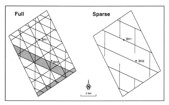
Fig. 3: Two selected geometric scenarios of the hybrid model: full- (left) and sparse scenario (right). BH1, BH2: location of existing deep boreholes
