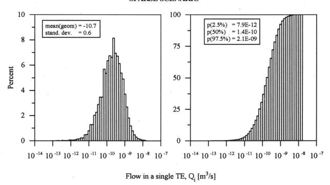
Fig. 6: Calculated distribution of volumetric flow in a single fracture, Q<sub>i</sub> [m<sup>3</sup>/s], full- and sparse scenario
