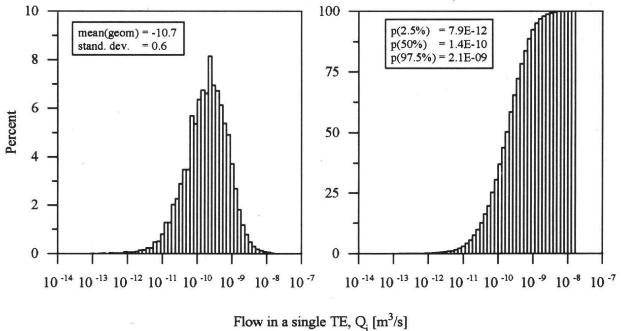
**Fig. 6:** Calculated distribution of volumetric flow in a single fracture,  $Q_i$  [ $m^3/s$ ], full- and sparse scenario
