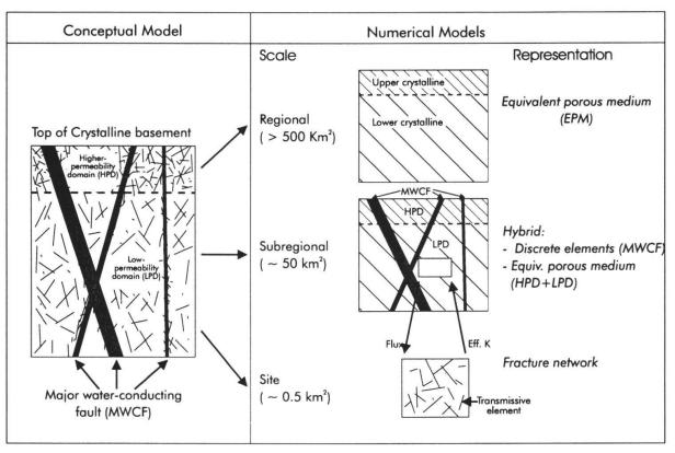
Fig. 2: Hydrogeological conceptual model and relationships to numerical models of groundwater flow
