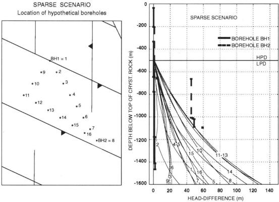
Fig. 4: Calculated vertical head profiles in hypothetical boreholes and comparison with experimental data in existing boreholes BH1 and BH2; full and sparse scenario
