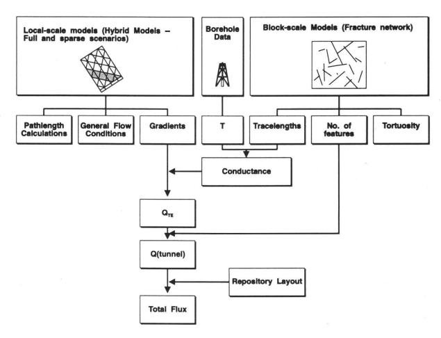
Fig. 5: Procedure for the derivation of the hydrogeologic input required for transport calculations
