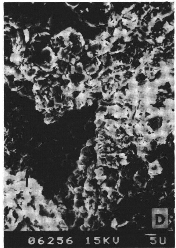
Fig. 4 - (a) Quartz overgrowth (OO) overlying Chlorit rim, scale bar 50 \mu\text{m} ; (b) Kaolinit (K) filling secondary porosity, note the vermicular form of the crystals; (c) Kaolinit as attacked pseudo-hexagonal plates and Chlorit (Ch) rim; (d) Chlorit rim in secondary pore space (see arrow).
