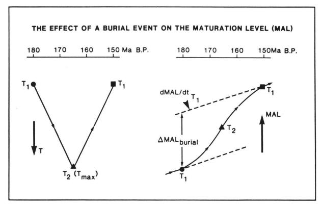
Figure 1: For the initial residence temperature (T<sub>1</sub>) the maturation level rises linearly with time. During the burial (heating) event maturation increses exponentially until maximum burial is reached (T<sub>2</sub>). During subsequent uplift (cooling) maturation decreases exponentially until the original temperature level (T<sub>1</sub>) is reached, after which it proceeds linearly at the original rate. A burial event produces a step in the maturation level of magnitude MAL.
