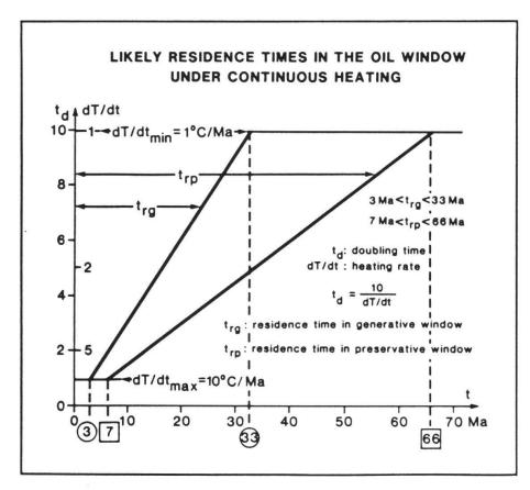
Figure 2: Here the likely residence times in the oil window are given for conditions of continuous heating (burial). It should be noted that the residence time in the generative window  $(t_{rg})$  and in the preservative window  $(t_{rp})$  can be rather short in what must be considered a normal geothermal environment.
