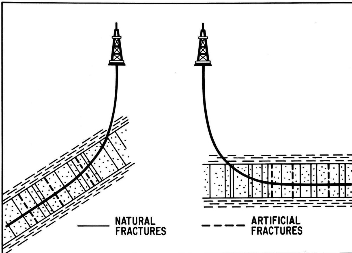
**FIGURE 6** The parallel completion technique combined with subsequent hydraulic fracturing. The azimuth of the deviation must be perpendicular to the open fracture set. A superior type of completion in any reservoir where macrofractures affect the fluid flow.
