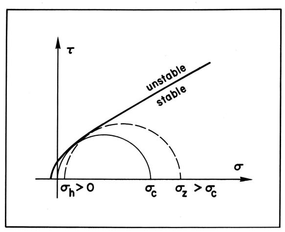
FIGURE 5 The concept of KING HUBBERT (1951): Where the effective overburden stress ( $\sigma_z$ ) exceeds the compressive strength of the rock ( $\sigma_c$ ) the minimum horizontal stress cannot be relaxed to a zero value without prior failure in shear (dashed circle).
