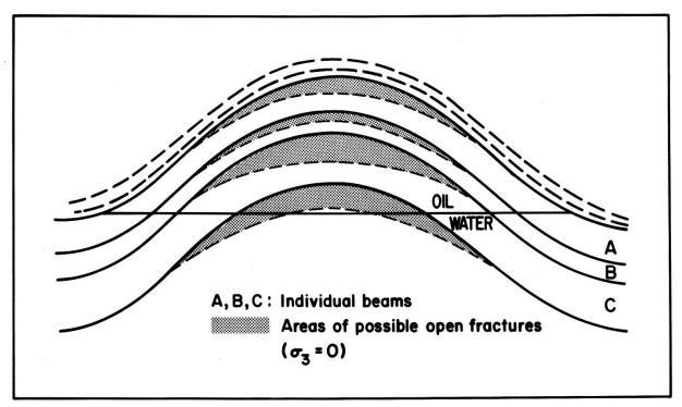
FIGURE 4 The expected distribution of fracture permeability and porosity in a multi-beam reservoir such as Ain Zalah. A real challenge to any EOR project.
