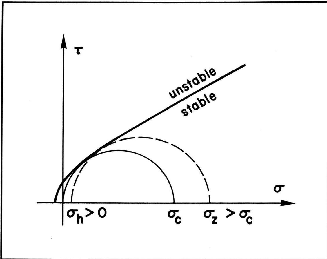
**FIGURE 5** The concept of KING HUBBERT (1951): Where the effective overburden stress ( $\sigma_z$ ) exceeds the compressive strength of the rock ( $\sigma_c$ ) the minimum horizontal stress cannot be relaxed to a zero value without prior failure in shear (dashed circle).
