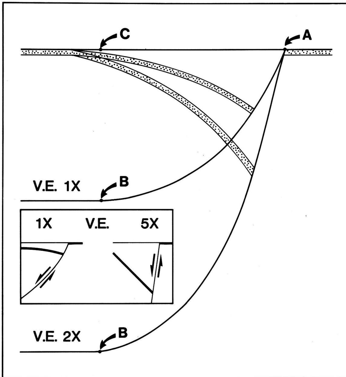
**Figure 2:** Vertical exaggeration has a highly destructive effect on cross sections containing normal faults. The roll-over is enhanced, the fault curvature reduced or eliminated and the structural style completely obscured.
