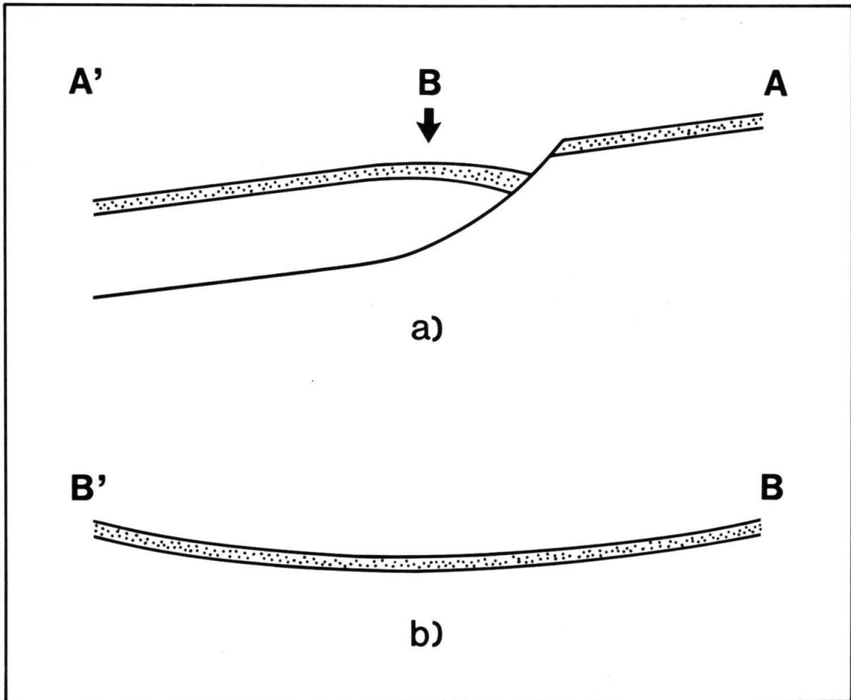
**Figure 4:** The down-dip (4a) and the strike (4b) cross sections for *Figure 3*. There is no closure in the strike direction and hydrocarbons will not be trapped as shown by their up-dip migration paths in *Figure 3*.
