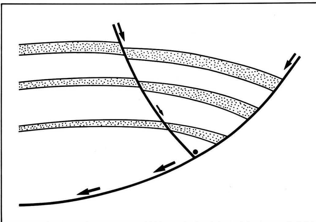
**Figure 7:** Extension is maximum at the surface (line AC in *Figure 6*). Antithetic faults, with displacement that is zero at the main fault and increases with distance from the sole fault, are the ideal mechanism to alleviate the variable extension experienced by the area ABC of *Figure 6*.
