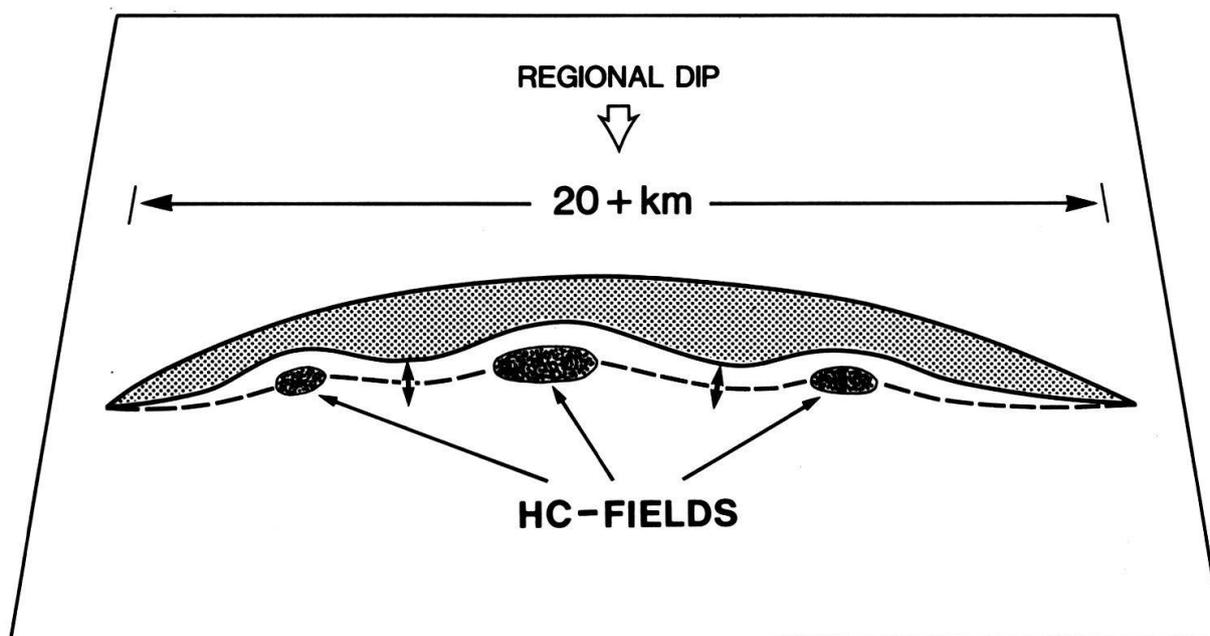
**Figure 5:** A giant regional growth fault superimposed on regional dip. Variable fault displacement may be sufficient to produce closed structures. In contrast to thrust faulting, axial culminations occur at locations of minimum fault displacement.
