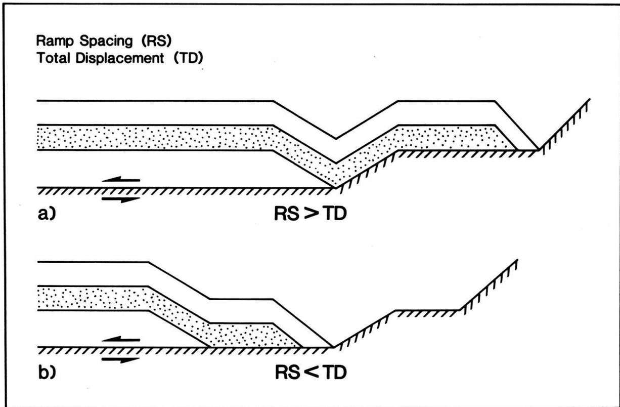
**Figure 8:** Schematic cross sections of structures formed above a listric fault containing multiple ramps. The resulting deformation is a function of the ramp spacing (RS) and the total displacement (TD).
