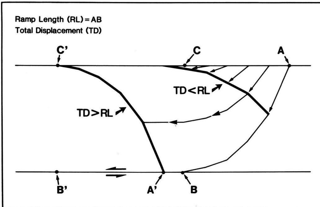
**Figure 6:** Deformation for the allochthonous sequence above a listric normal fault is restricted to the area ABC. For a total displacement (TD) exceeding the ramp length (RL) no further deformation occurs since behind line BC only layer parallel gliding occurs. Roll-over and fault curvature are related and line A'C' is the displaced mirror image of line AB. Curvatures are approximated by straight line segments and no allowance is made for contemporaneous sedimentation.
