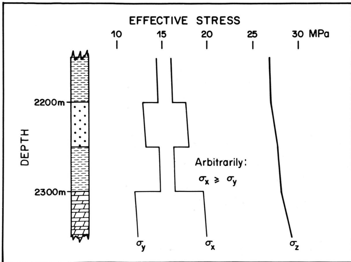
Fig. 5 A schematic view of the effective principal stresses in a layered sedimentary sequence. The effective overburden stress ( $\sigma_z$ ) is a continuous function of depth. This is NOT the case for the principal lateral effective stresses ( $\sigma_x$  and  $\sigma_y$ ) which must change abruptly at bedding planes separating different lithologies. This is true for all tectonic realms, be it compression, extension, or simple gravitational loading.
