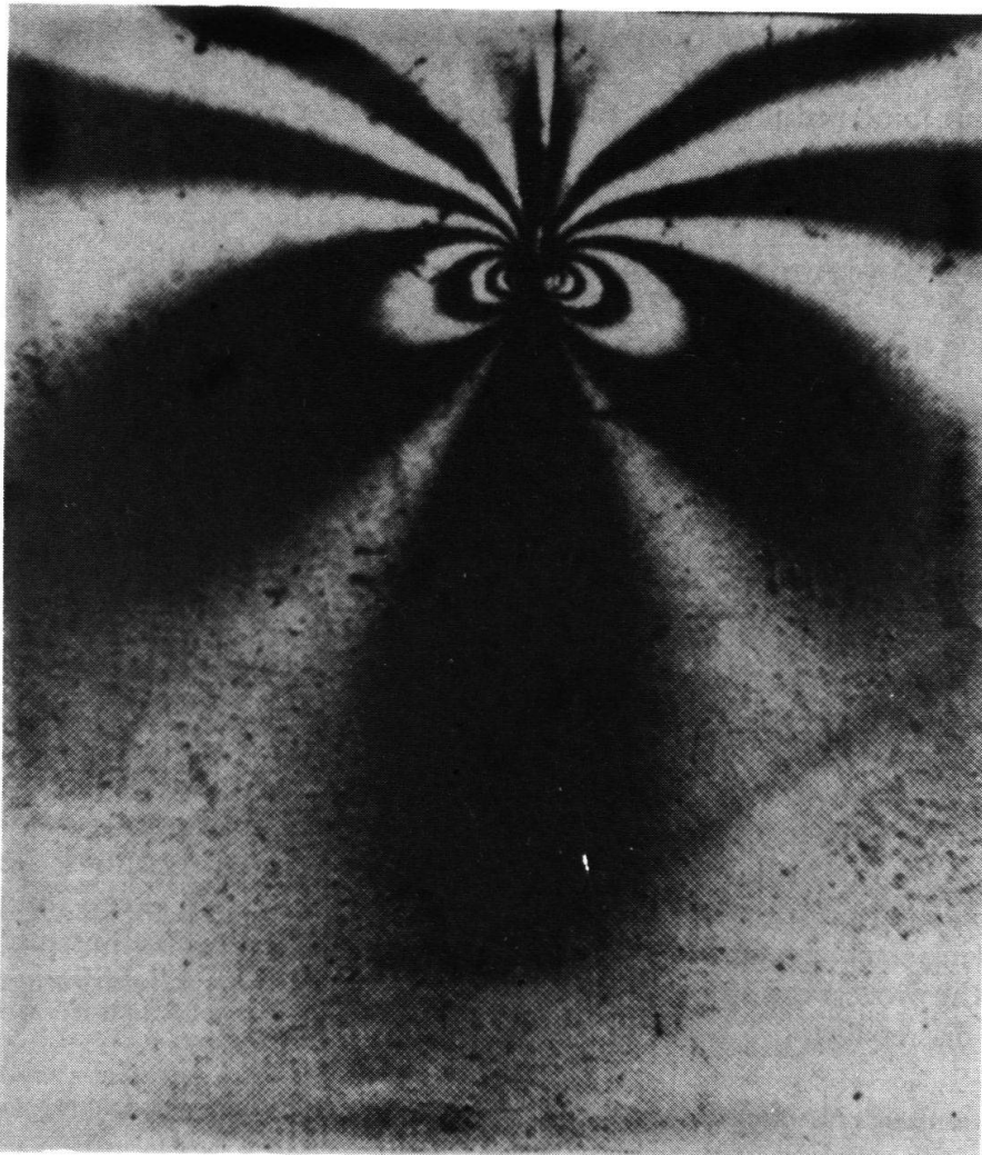
Fig. 1 Stress concentration at the tip of an open fracture as seen in a photo-elastic model.
