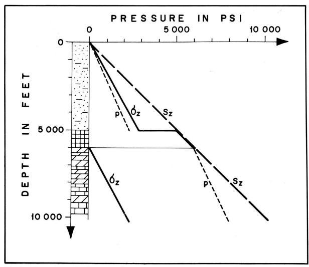
Fig. 1 The total overburden stress  $(S_z)$ , the pore pressure (p), and the effective or matrix overburden stress  $(\sigma_z)$  in a sedimentary sequence containing a perfect seal such as a salt layer. Note that:  $S_z = \sigma_z + p$  or for  $p = S_z$  such as directly below the salt we have:  $\sigma_z = 0$ , i. e. no stress in the rock matrix. (from GRETENER, 1969)
