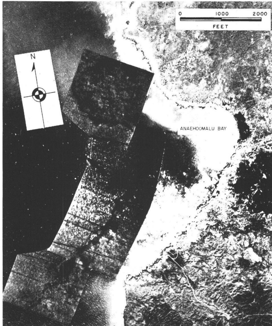
Fig. 11: Infrared images mounted on an aerial photograph of Anaeheomalu Bay (Hawaii). The thermal anomaly produced by groundwater outflow is indicated by black arrow (from ADAMS et al.).
