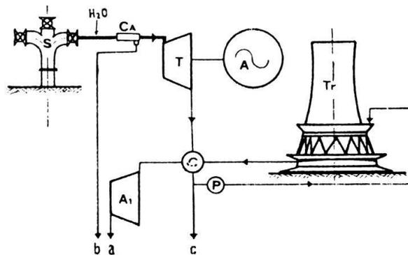
Fig. 5: Condensing geothermal plant, Larderello (ENEL, 1970).
