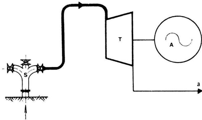
Fig. 4: Non-condensing geothermal plant, Larderello (ENEL, 1970).
