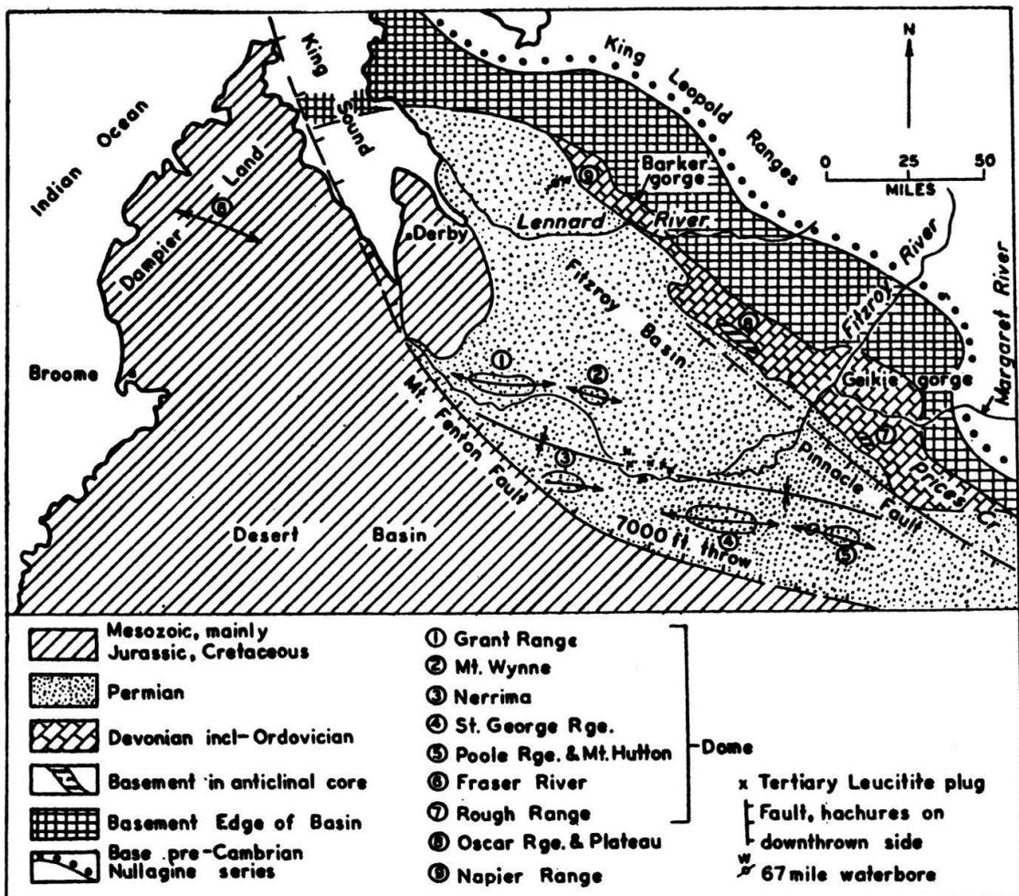
Fig. 4 — Fitzroy-Canning Basin, Western Australia, Structural Interpretation prior to Drilling (after SCHNEEBERGER in World Oil, 1954).
