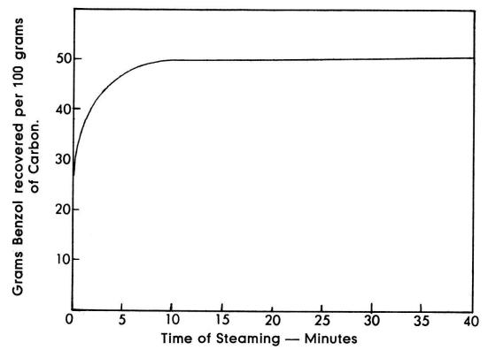
Fig. 2. Desorption of Benzol by Wet Steam. Benzol Held by Carbon at Saturation, 57 % by Weight (Ray).
