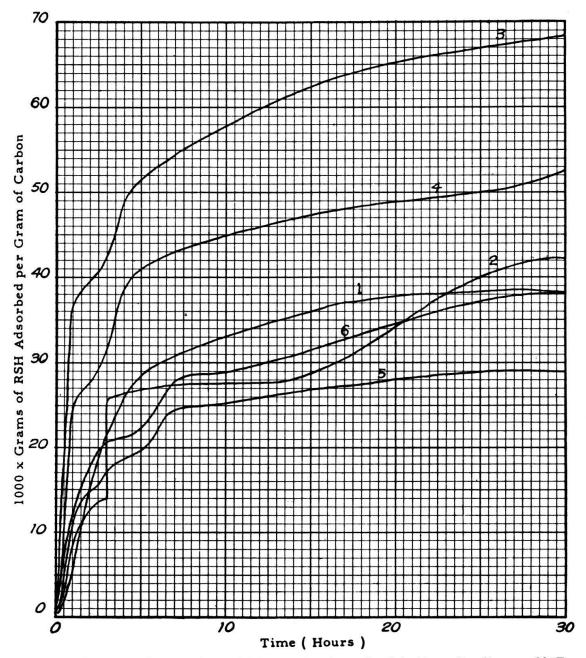
Fig. 4. Rate of extraction of Mercaptans from Straight-Run Gasoline at 830 F. (Curve 1, n-Propyl; 2, iso-Propyl; 3, n-Butyl; 4, iso-Butyl; 5, tertiary Butyl; 6, n-Amyl (Courtesy Petroleum Refiner).
