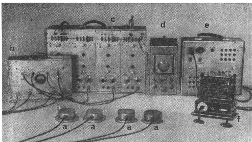
Fig. 3 Four-canal accelerometer
