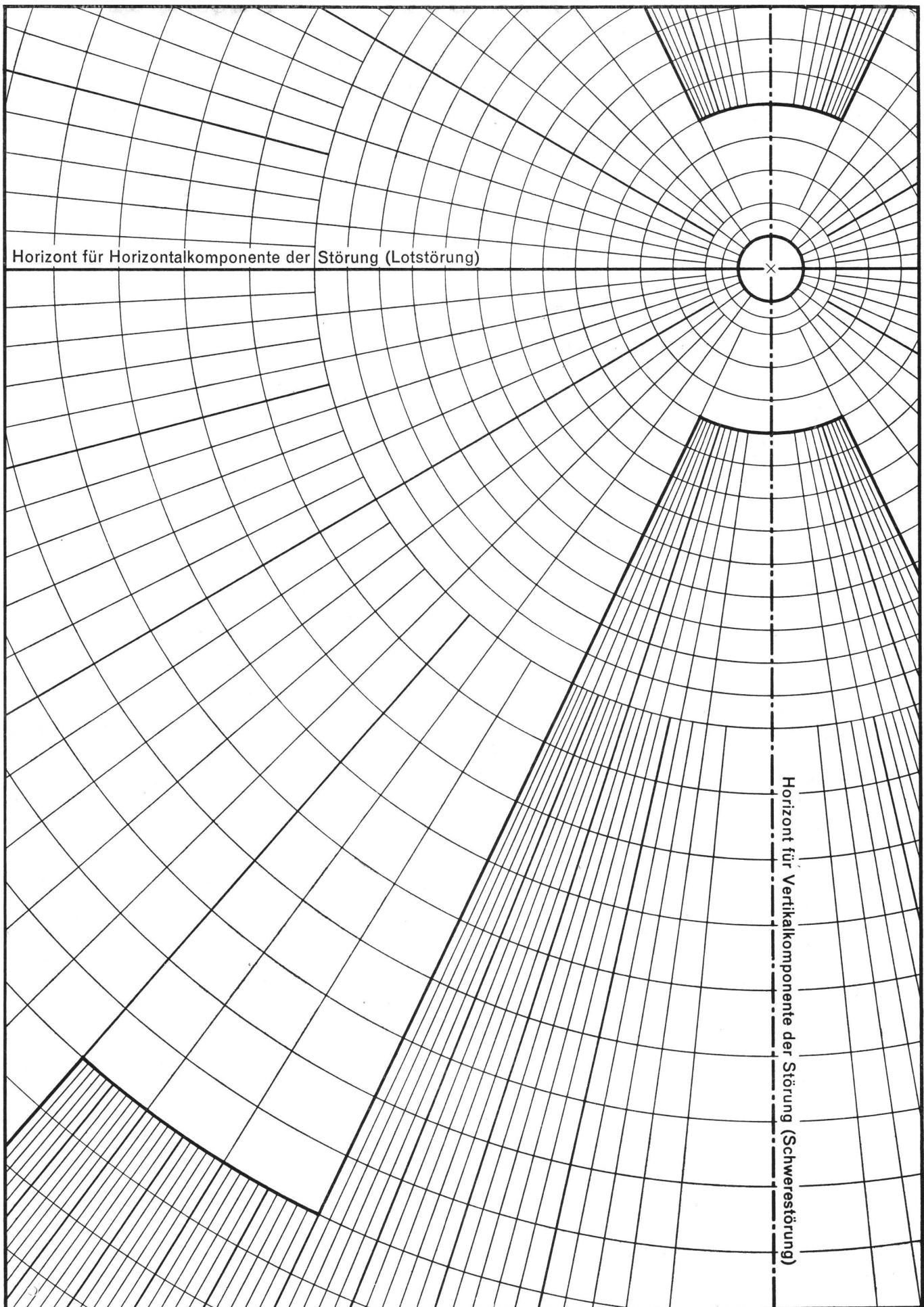
late 1 Part of a diagram for the graphical computation of attraction due to «two-dimensional» masses (from K. Jung, modified).
