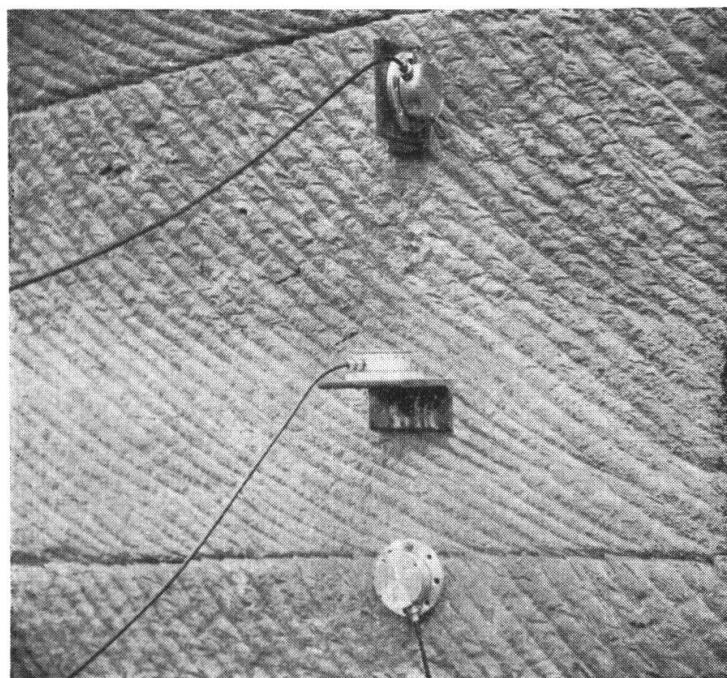
Fig. 7 Three accelerometers tacked on a sandstone-wall
