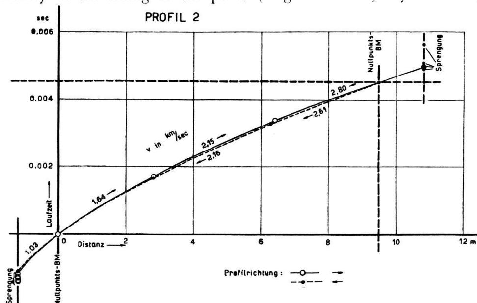
Fig. 5 Travel time curves, taken in two opposite directions
