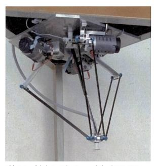
Abb. 1. Parallelroboter Delta, Reymond Clavel, EPFL 1986.
