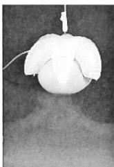
Figure 5. Soft robotics in action. Compartments made from a silicon-based polymer are filled with air. As the sides of the compartments have different wall strengths, the application of air will lead to a reversible deformation of the material. The six-legged star-shaped polymer is forced into a bent conformation and can grip a raw egg without crushing it. Reprinted with permission from Angewandte Chemie International Edition 2011, 50, 1890–1895. Copyright 2011.
