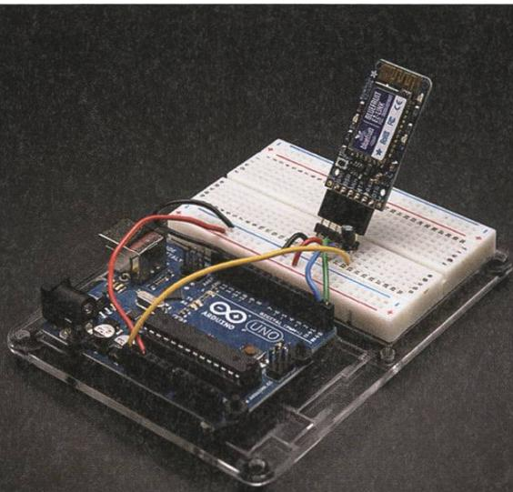
BLE module with Arduino
