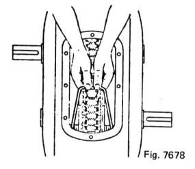
Press down and lift up chain and shoe assembly.
