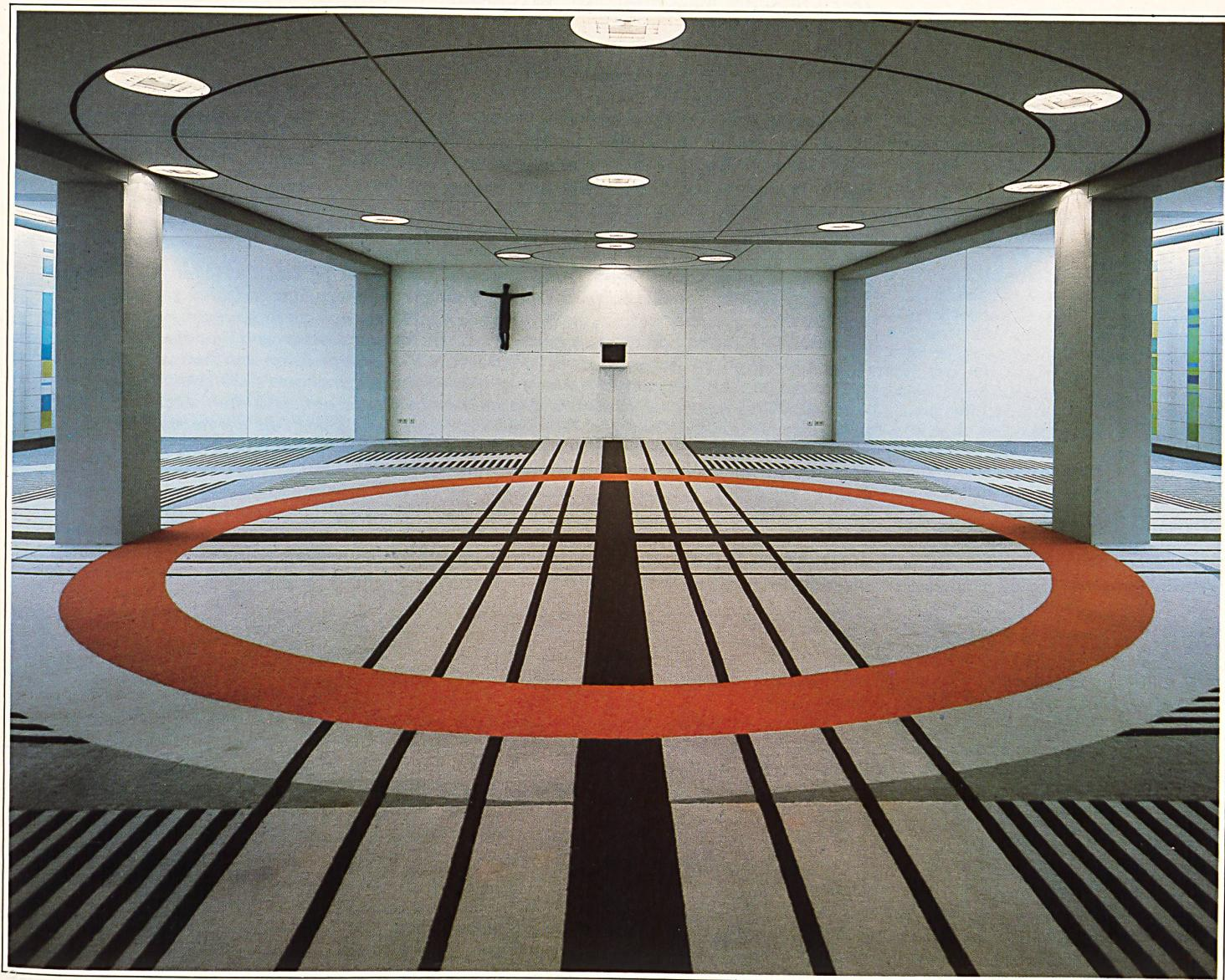
■ "Waron" carpets are neither woven nor tufted but produced on converted embroidery machines according to a manufacturing process developed by Walter Nüesch. Each carpet is a one-off production made individually and exactly to measure, to fit any shape of room. Over 100 standard colours are available to choose from, but special colour requirements are also executed for orders of over 5 m<sup>2</sup>.
