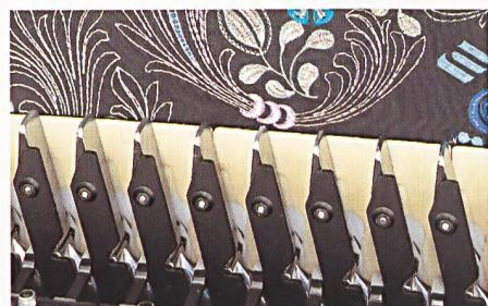
Pentacut thread cutting device on the shuttle side.
