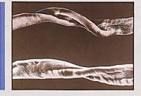
A single fibre under the scanning electron microscope. Cotton is eminently suitable for spinning both because of its fineness and because of its corkscrew-shaped coils.
