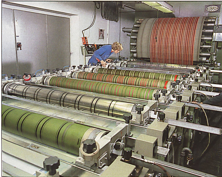
Up to 14 colours can be applied over a fabric width of 180 cm by this rotary screen-printing machine.
