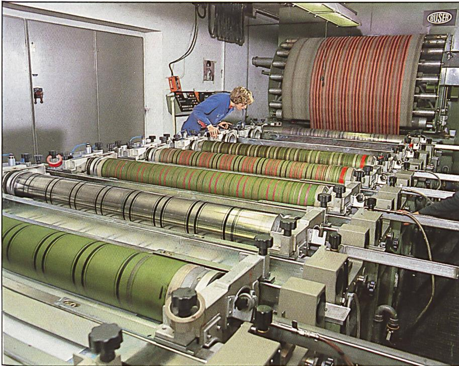
Up to 14 colours can be applied over a fabric width of 180 cm by this rotary screen-printing machine.
