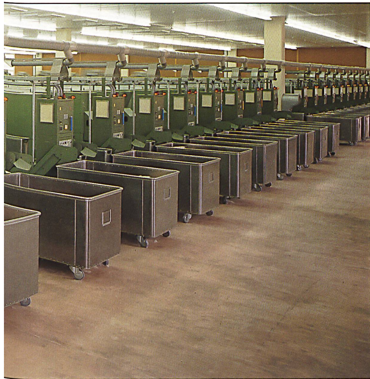
Profitability has been boosted remarkably by these new ring spinning frames with incorporated Rieter doffer.
