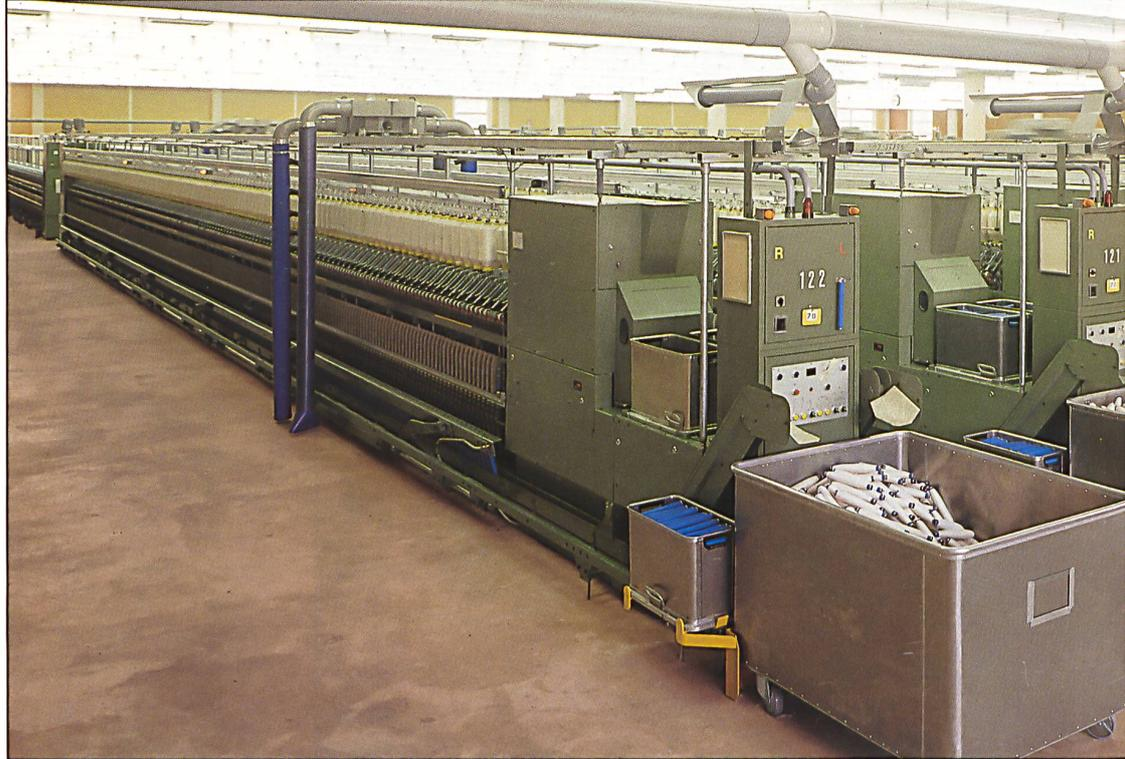
*An ultra-modern plant: The spaci-ously designed spinning room houses fully automatic ring spinning frames.*
