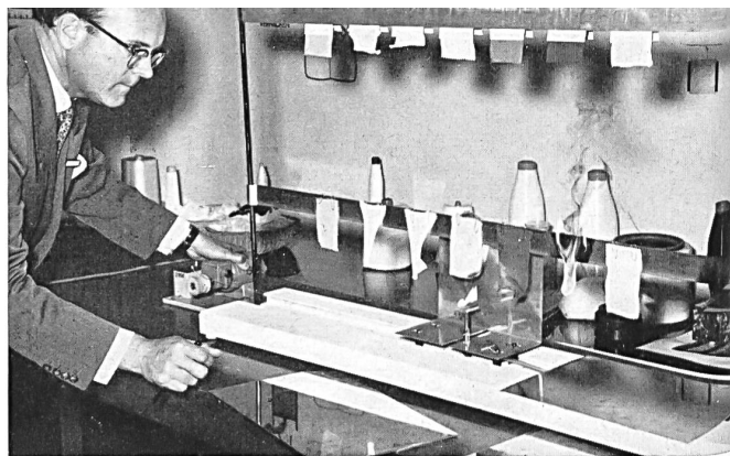
Testing the inflammability of different textile samples.
