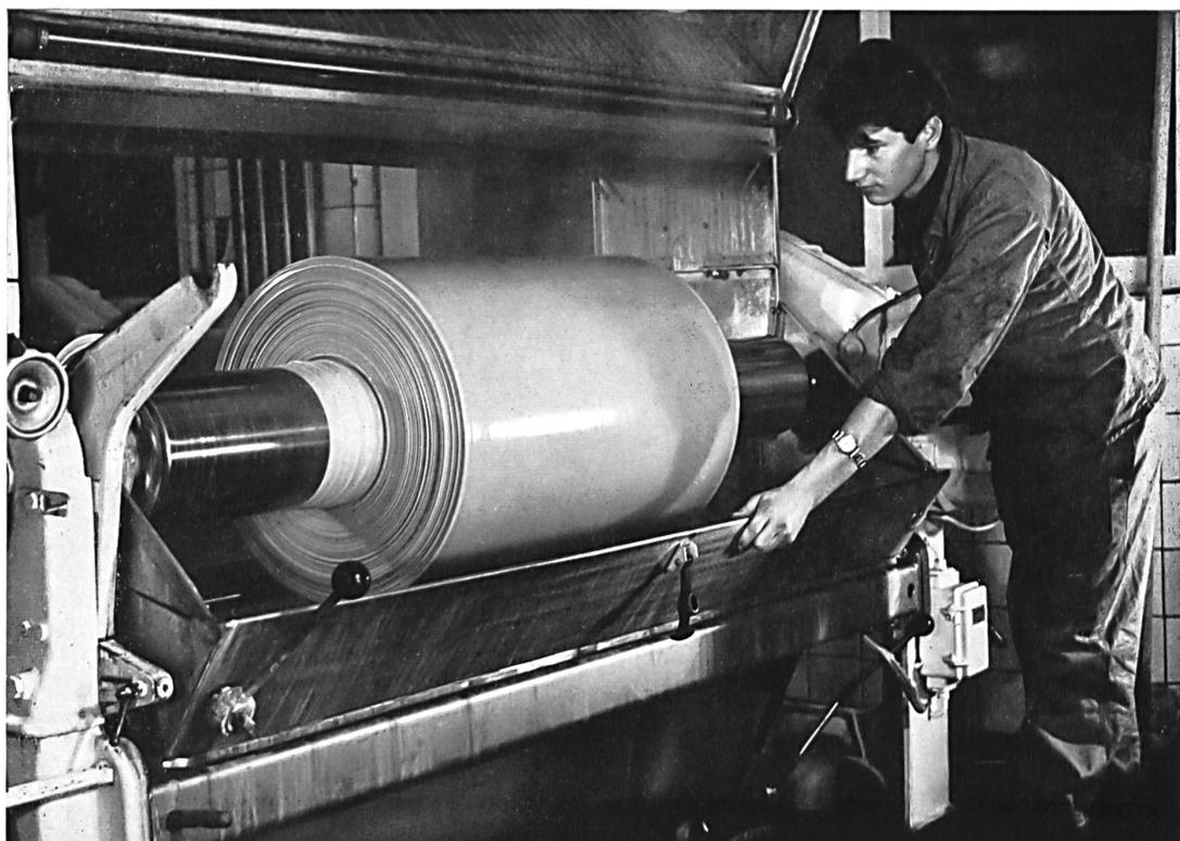
Piece dyeing on an automatic jigger
