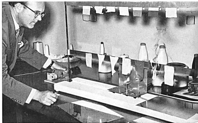
Testing the inflammability of different textile samples.
