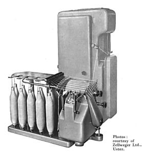
« Uster » yarn strength tester with automatic multiple-bobbin attachment.
