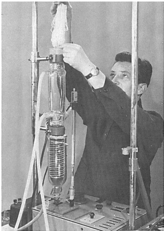
Dyeometer for measuring the time required by the textiles to absorb the dye in the bath.
