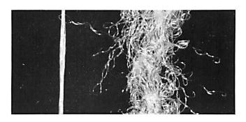
On the left, untreated nylon yarn; on the right, the same yarn after the treatment which has transformed it into a Helanca yarn (magnification 40 x).
