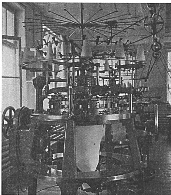
Cotton's knitting machine for knitting stockings, named after the inventor, possesses as many as 32 different appliances called needle-beds. On this machine fashioning is automatic which makes it possible to manufacture fully fashioned stockings.
