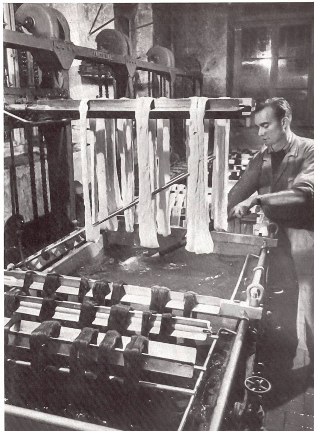
Hank dyeing machine for silk twists.
