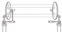
Fig. 307 Reflection of sound waves radiating from a source (pocket watch) at the surface of a concave mirror surface
