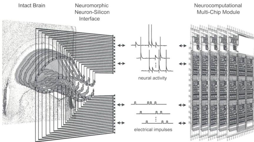
fig 7: Brain prosthesis, a neuromorphic interface connects the intact neural tissue to the chip module.
