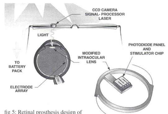
fig 5: Retinal prosthesis design of Harvard/MIT research group.
