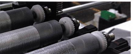
Abb. 1: Positive Patternbeam Drive (PPD)
