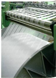
Abb. 5: DIGICAST Kettfadentransport
