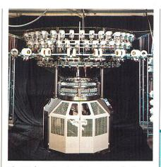
The SJE from Camber International's SJ range of machines ofer 3-way technique. Die Rundstrickmaschine SJE von Camber International bietet 3-Wege-Technik
