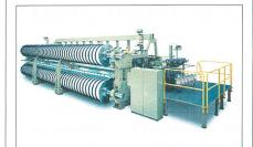
Sulzer Textil Projectile Weaving Machine for forming fabrics – 8.46 m wide weighing some 45 to 50 metric tons
