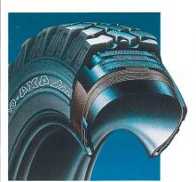
The structure of a radial tyre consists of fabric layers that are arranged radially and diagonally to the tyre axis
