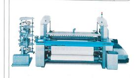
Sulzer Textil Airjet Weaving Machine – weaving glass fibre yarns
