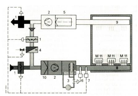
Condifil Klimasystem, M = Textilmaschine, I = Regelklappe, 2 = Ventilator, 3 = Luftwäscher, 4 = Lufterhitzer, 5 = Abluftfilter, 6 = Feuchtefühler, 7 = Temperaturfühler, 8 = Zuluft, 9 = Abluft Grafik: Sulzer Infra
