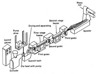
Figure 3. Schematic of monofilament extrusion line.
