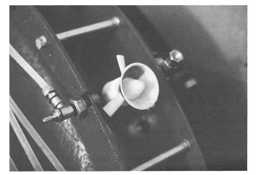
Buse rotative X<sub>1</sub> de Micron Sprayers.
