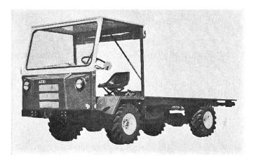
Fig. 4: Char automobile (transporter) AEBI TP 35, charge utile 2200 kg.
