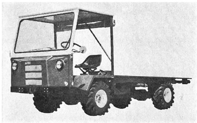
Fig. 4: Char automobile (transporter) AEBl TP 35, charge utile 2200 kg.
