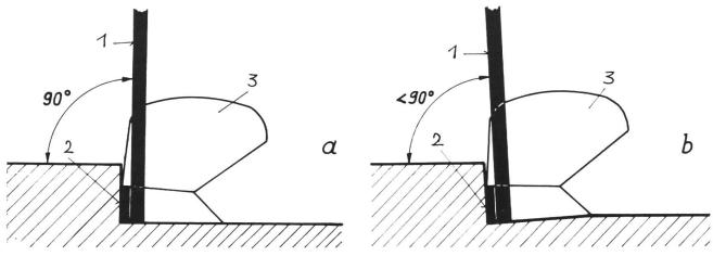
Fig. 13: 1 = Etançon supportant le corps de charrue 2 = Talon 3 = Corps de charrue
