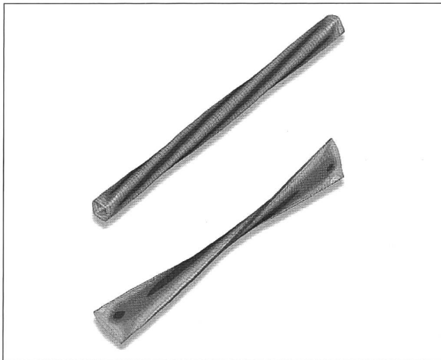
Figure 5: Free deformation of fibers during drying.
