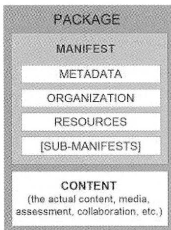
Figure 1: LO Physical Structure (taken from IMS, 2005)
