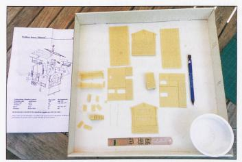
3. Remove casting block remains, wash, dry.
