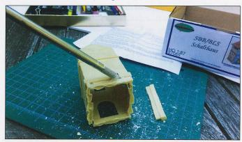
Step 3 - Carefully remove the casting blocks.
