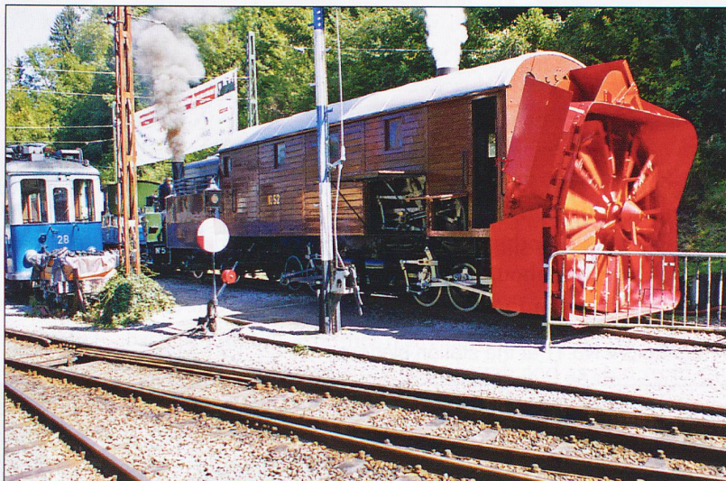
RhB No.9214 Xrotd 6/6 rotary snow plough, with the plough rotating, hence the railing in front.
