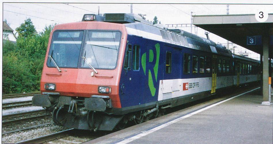
1. SBB ‘Domino’ unidentified driving trailer at Ligerz on 27 October 2017. Note the MU cable fitted to units without automatic couplers.
