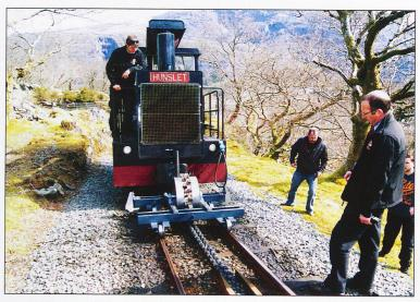
During April 2016 the Swiss Team made gauging trials with the 'Brienz Roller'. Under the guidance of Mike Robertshaw (nearest camera), we were able to determine exactly where our limits of running are. This photo shows the commencement of the Gripper Rail which, as suspected lies foul of the Brake Drums, simulated by the two round rings left and right of the Pinion Wheels.
