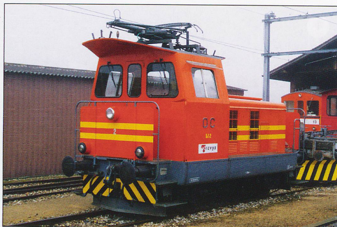
Travys (ex Orbe Chavornay) shunting loco Ee2/2 No. 2 in Orbe showing old and new branding.
