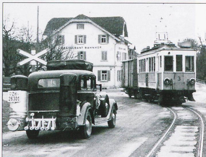
A car fitted with a 'Producer Gas' generator ,waits for UOe CFe 2/2 No.3 to leave Esslingen for Oetwil. 1946.
