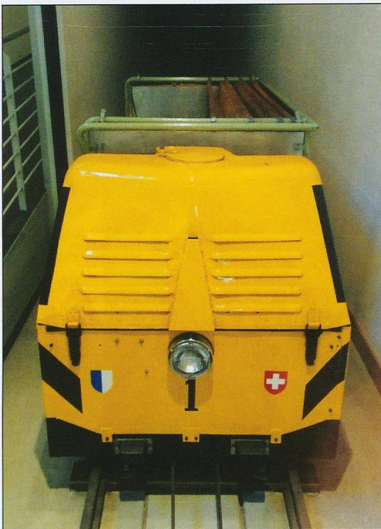
main station floor. Operation of the railway was very simple using push buttons as in a lift. With these buttons the car could be sent to the other end, or called from there. To prevent the car from being called to the other end while being loaded, gates were installed that had to be closed to permit movement.
