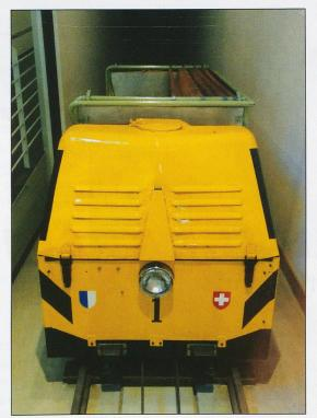
main station floor. Operation of the railway was very simple using push buttons as in a lift. With these buttons the car could be sent to the other end, or called from there. To prevent the car from being called to the other end while being loaded, gates were installed that had to be closed to permit movement.
